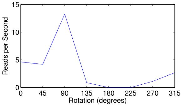
Figure 10. Occlusion due to the body at 2 meters
